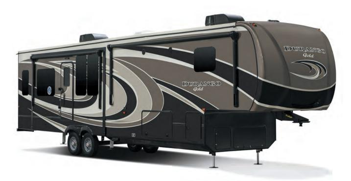
leaves 2,745 pounds of cargo carrying capacity. (My test unit, with several options, weighed 12,360 pounds.) Because this model is designed for full-time use, it's not a lightweight trailer and will require a one-ton truck to tow safely, although some <sup>3</sup>/<sub>4</sub>-ton trucks may handle it.
