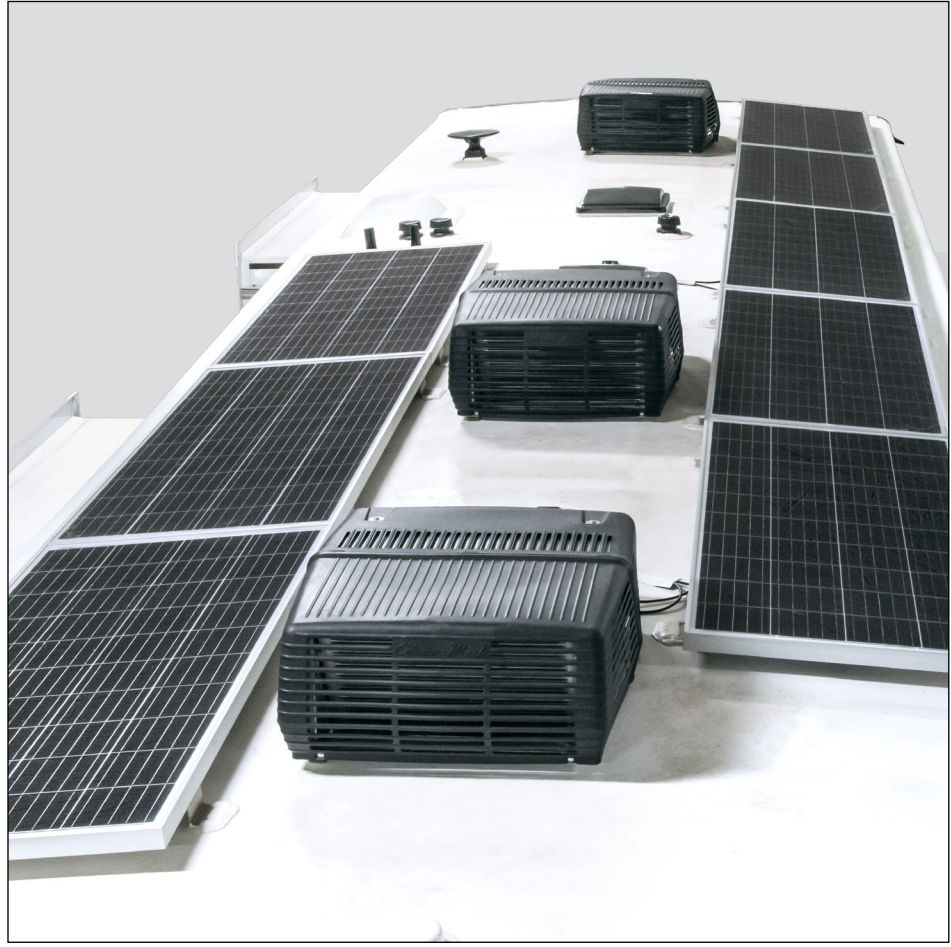
(8) 220W solar panels = 1,760 Watts of solar power
