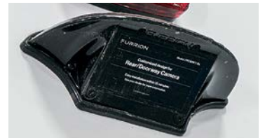
BACKUP CAMERA PREP ready for wireless observation camera system
