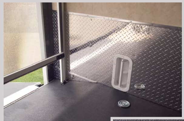
Track Mounted Roll Down Insect Screen (optional), Side Wall Mounted Venting, Side Wall Diamond Plate, Dove Tail Rear Ramp Entry Detail with Tuff Ply Coating and 9 Tie Down Rings.
