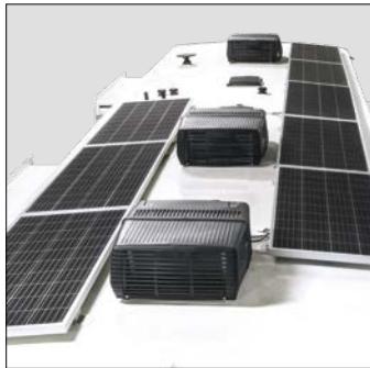
(10) 200W solar panels = 2,000 Watts of solar power
