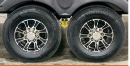
Nitrogen-filled 16-inch tires with ALUMINUM WHEELS, spare tire and self-adjusting brakes. Equa-Flex rubberized equalizer absorbs road shock and reduces fore-to-aft movement.
