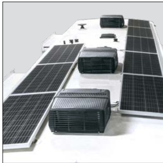
(8) 220W solar panels = 1,760 Watts of solar power
