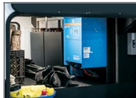
Optional Boondocker Solar system - a 48V marvel that starts w/ (8) 220W panels, (2) 200AH 48V LI batteries, 5,000W Inverter (Powers everything inc 1 A/C), plus a list of class leading Victron components!
