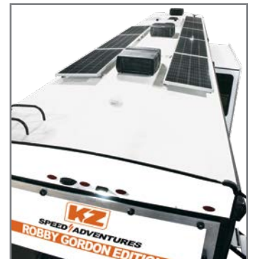
Optional Boondocker Solar system - a 48V marvel that starts w/ (8) 220W panels, (2) 200AH 48V LI batteries, 5,000W Inverter (Powers everything inc 1 A/C), plus a list of class leading Victron components!
